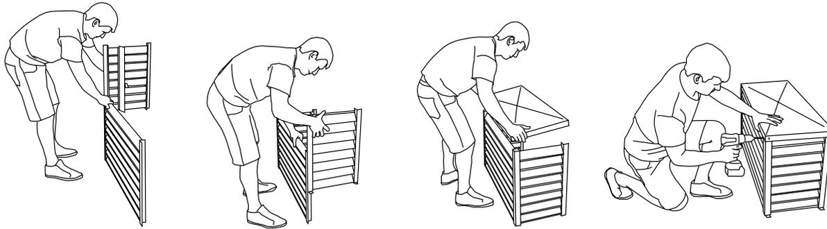
Tools required are a square drive screwdriver for assembly and a drill and driver for the anchor fixings which can vary depending on the material you are fastening to.
